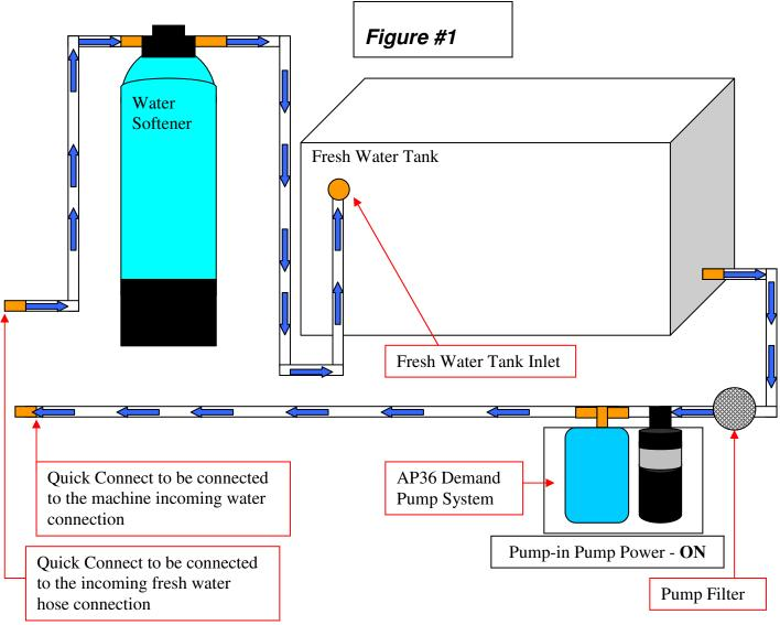
When installing a water softener with a fresh water tank, the water softener should be placed on the fill or incoming side of the fresh water tank and its water flow path. The softened water from the fresh water tank will flow to the Pump-in pump and be pumped to the incoming water connection on the front of the machine. (See Figure #1)
